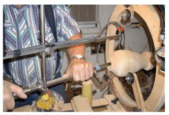
Hollowing of a deep vessel
