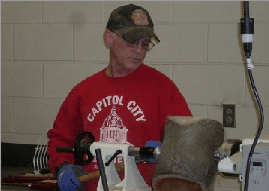
The blank is mounted crosswise in the lathe. Drive is from a spur center recessed into the blank.
