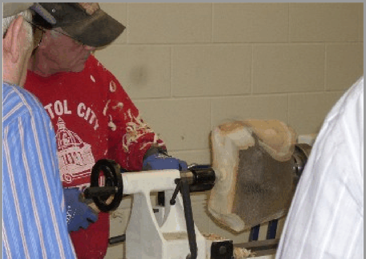
Frank making initial cuts on what will be the base of the bowl.
