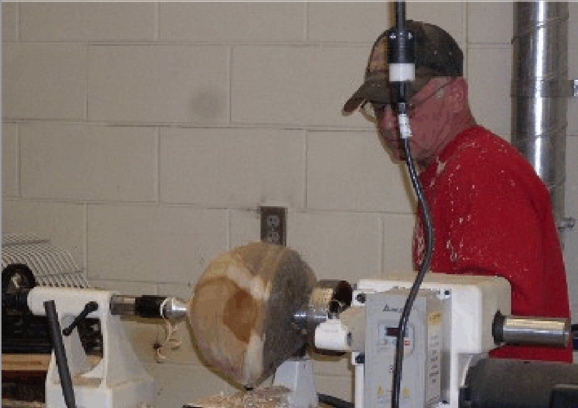
The lower portion of the bowl has taken initial form and a tenon or recess has been turned to facilitate holding when the blank is reversed.
