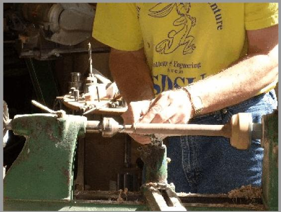
A bead is rolled next to the tenon on the end of the spindle. The other end of the square blank is driven in a shop made socket on a small faceplate.
