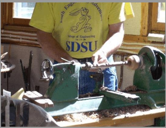
The rest of the spindle takes shape. These are good pieces to learn shearing cuts to minimize the amount of sanding. Hate that sanding....
