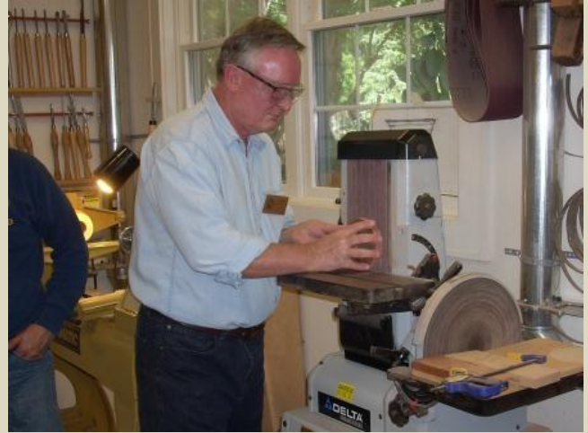
Flattening a ring on the belt sander
