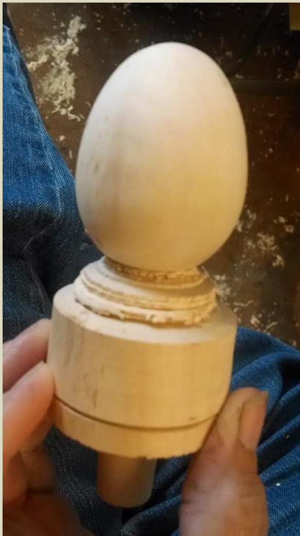
One of Alan Lacer's favorite projects to hone and test one's skills with a skew chisel is turning wooden eggs.
