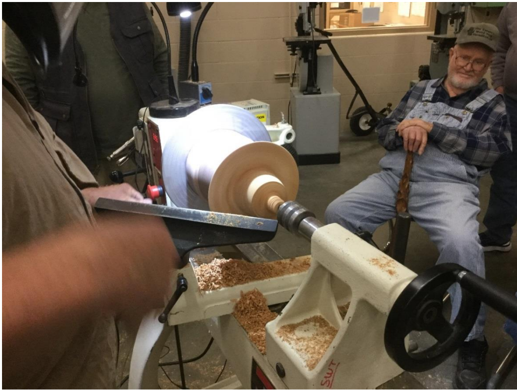
The outside of the crown nearing completion.
