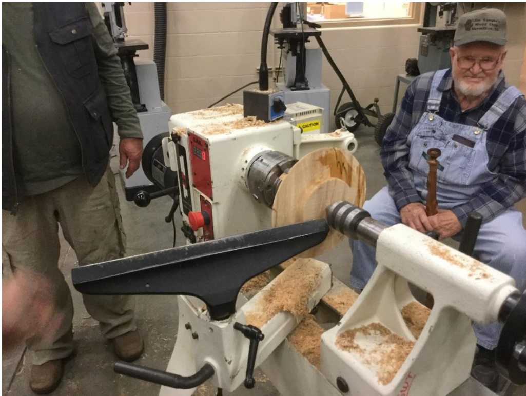
The blank reversed and mounted in the chuck for hollowing of the crown of the hat and finishing of the brim.
