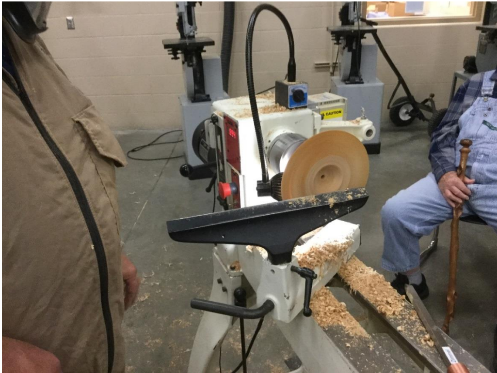
Light mounted to show the thickness of the crown and the brim as they completed
