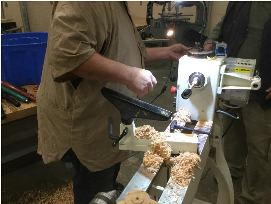
That's right! You are seeing a light socket installed through the headstock. The light will be used to show the thickness of the upper part of the crown as it is finished while mounted on the special chuck jaws in the next picture.
