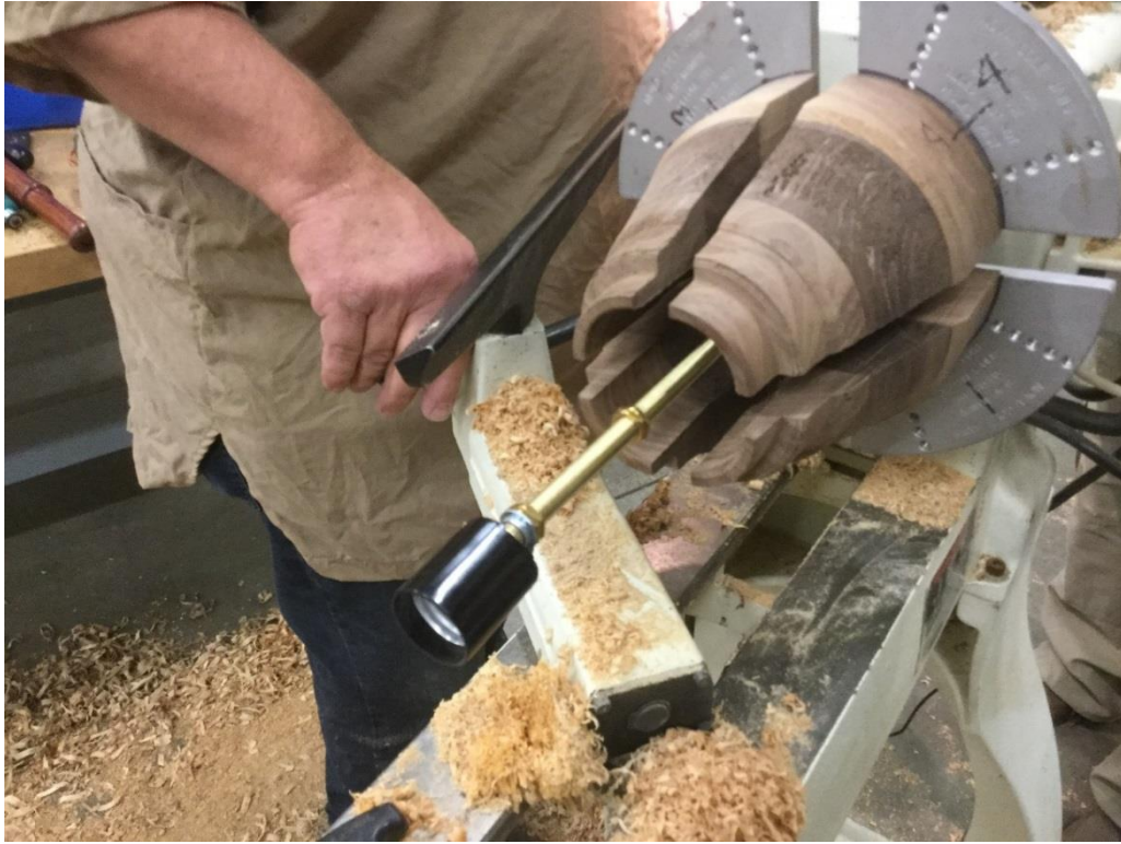
Preparing to mount the hat on the special chuck jaws. The light socket will be positioned inside these jaws when the blank is again reversed and mounted.
