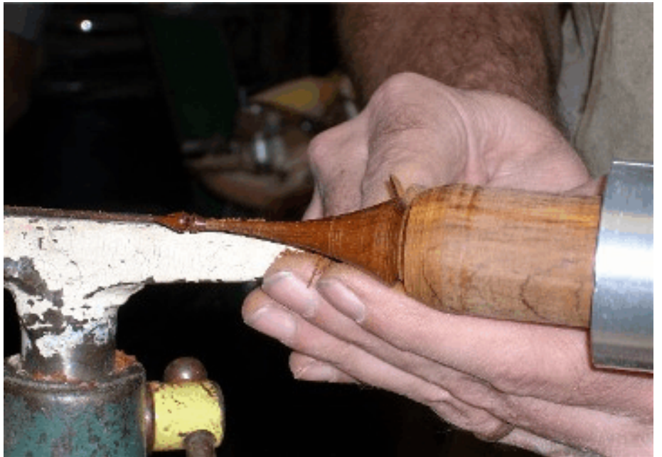
Turning the finial for an ornament. Best place to learn how to use a skew chisel.
